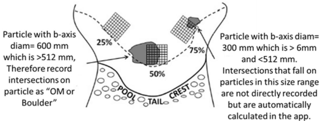
**Figure G2.** Adapted from PIBO. Record intersections of the fines grid that land on particles 512 mm (b-axis diam. as “OM or boulder”). Do not record the number of intersections that fall on particles > 6mm and <512 mm.
