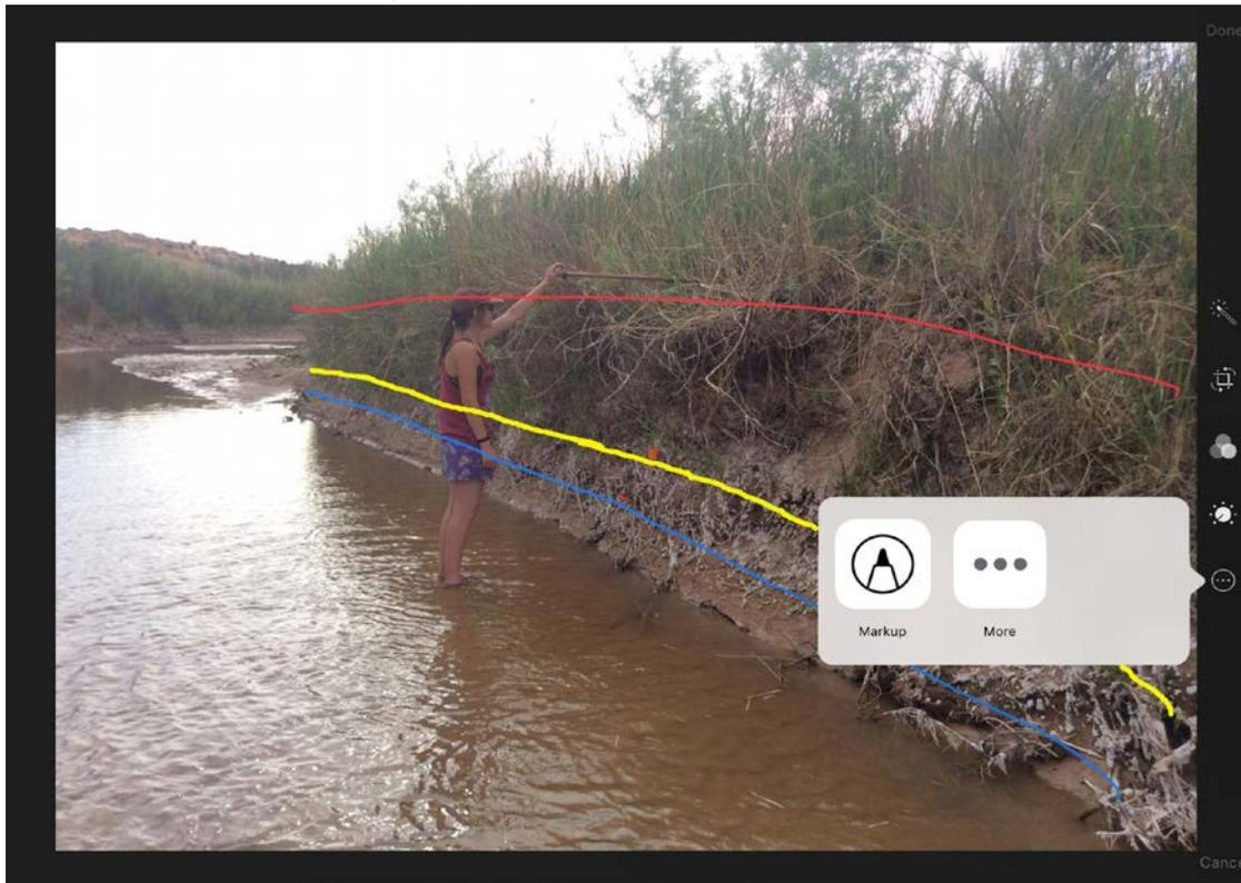
**Figure 31.** Example critical concepts photo with lines drawn on the photo to indicate scour (blue), bankfull (yellow), and floodplain (red) features. Note the markup tool in the iPad photos application can be used to draw these lines and then the photo should be uploaded into the SARAH application.
