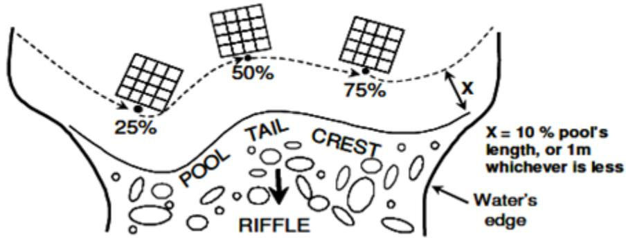
**Figure G1.** Adapted from PIBO. Location and orientation of the pool tail fines grids relative to the pool tail crest
