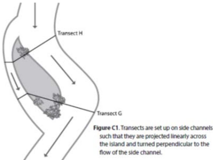
Figure C1. Transects are set up on side channels such that they are projected linearly across the island and turned perpendicular to the flow of the side channel.
